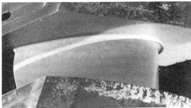
Fig. 11 Suction surface and outer platform flow visualizations
